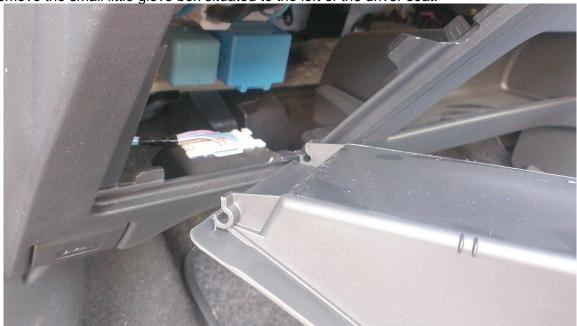
Note the flasher relay is the big unit from the bottom right of the panel:
