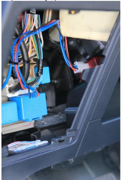
Attach the module to the top of the plastic board below the steering wheel:
