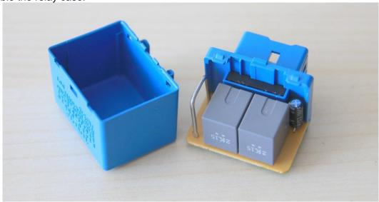
To remove the PCB from the socket, you need to pull the black little blocker plastic:
